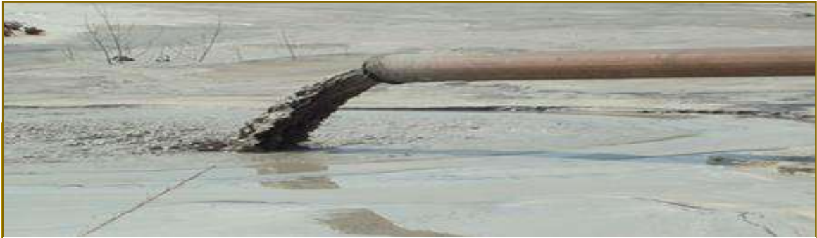
Figure 3: Lean Slurry Disposal System
